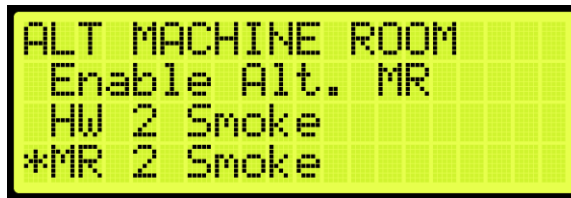
Figure 573: ALT MACHINE ROOM Menu – MR 2 Smoke
