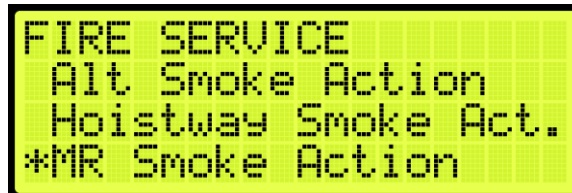
Figure 547: FIRE SERVICE Menu – MR Smoke Action
