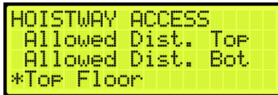
Figure 402: HOISTWAY ACCESS – Top Floor
