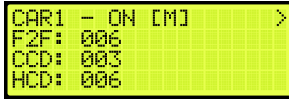
Figure 275: Dispatching Timers Status
