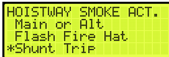
Figure 545: HOISTWAY SMOKE ACTION Menu – Shunt Trip
