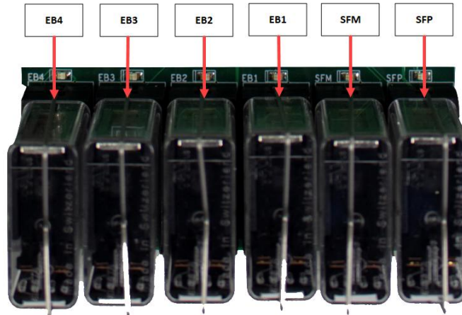
Figure 23: MR Board SR3032 Safety Relays
