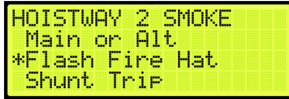
Figure 570: HOISTWAY 2 SMOKE Menu – Flash Fire Hat
