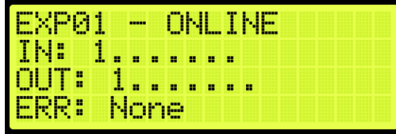
Figure 610: Active Expansion Board Status
