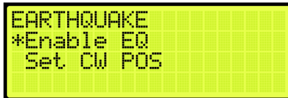
Figure 508: EARTHQUAKE Menu – Enable EQ
