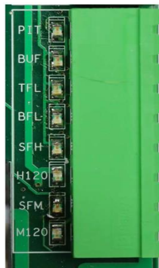
Figure 19: Safety String Input Connector
