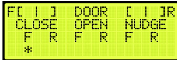
Figure 673: Enter Door Command Menu (Front and Rear Doors)
