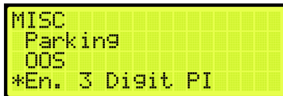
Figure 446: MISCELLANEOUS Menu – Enable 3 Digit PI
