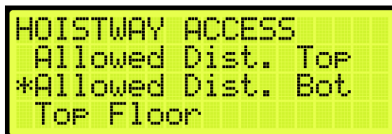
Figure 404: HOISTWAY ACCESS – Allowed Distance Bottom
