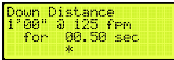
Figure 355: Down Distance Menu – Steady State of Leveling Longer Adjustment
