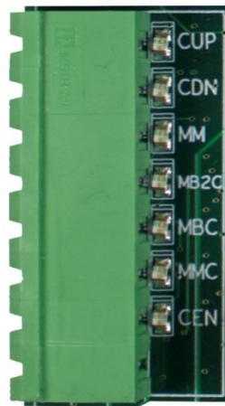
Figure 18: 24 VDC Monitoring System Connector
