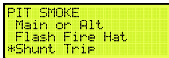
Figure 560: PIT SMOKE Menu – Shunt Trip
