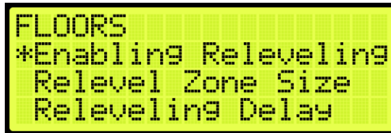
Figure 149: FLOORS Menu – Enable Releveling
