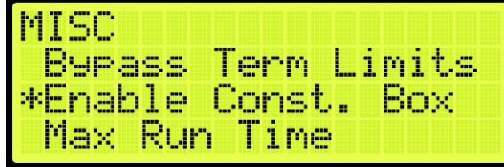
Figure 416: MISCELLANEOUS Menu – Enable Construction Box
