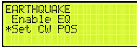
Figure 510: EARTHQUAKE Menu – Set CW POS
