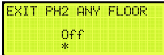
Figure 586: EXIT PH2 ANY FLOOR Menu
