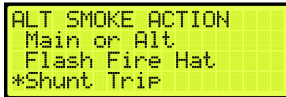
Figure 536: ALT SMOKE ACTION Menu – Shunt Trip
