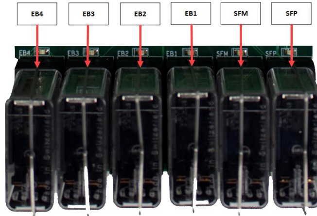
Figure 23: MR Board SR3032 Safety Relays
