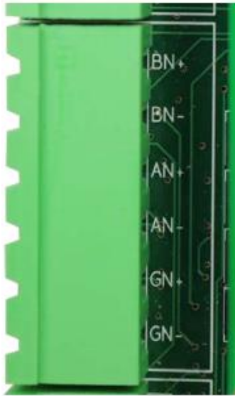
Figure 14: CAN 1,2,3 Network Connector
