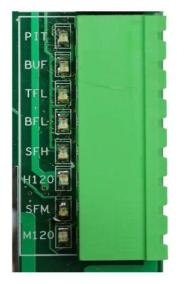
Figure 19: Safety String Input Connector
