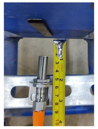
Figure 117: Mounting Proximity Sensor Assembly (Example)
