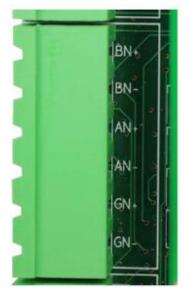
Figure 14: CAN 1,2,3 Network Connector
