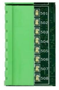
Figure 16: 24 VDC Input Connector
