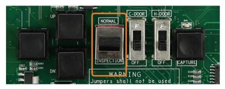
Figure 78: MR INSPECTION Switch
