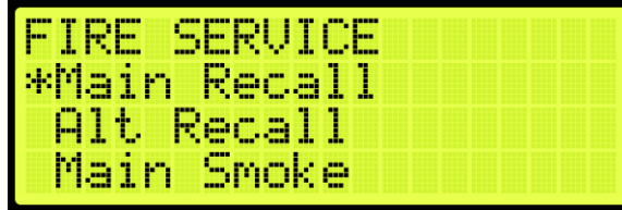
Figure 559: FIRE SERVICE Menu – Main Recall
