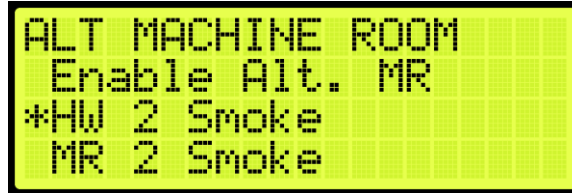
Figure 610: ALT MACHINE ROOM Menu – HW 2 Smoke
