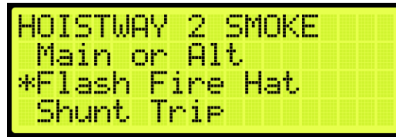
Figure 613: HOISTWAY 2 SMOKE Menu – Flash Fire Hat
