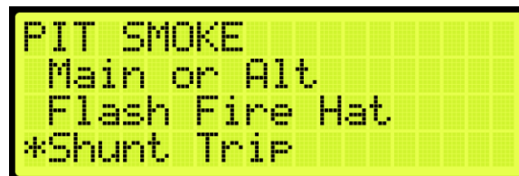
Figure 605: PIT SMOKE Menu – Shunt Trip
