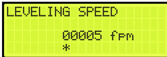
Figure 219: LEVELING SPEED Menu
