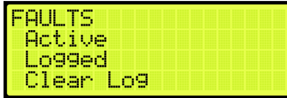
Figure 52: FAULTS Menu – Active, Logged, Clear Log
