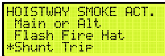
Figure 588: HOISTWAY SMOKE ACTION Menu – Shunt Trip
