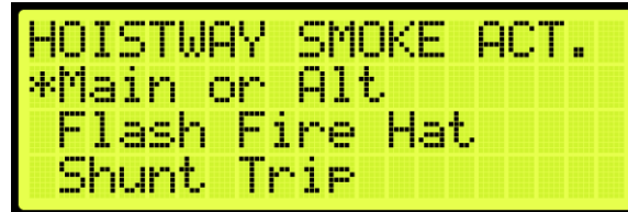
Figure 584: HOISTWAY SMOKE ACTION Menu – Main or Alt
