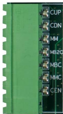
Figure 18: 24 VDC Monitoring System Connector
