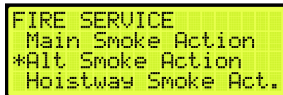
Figure 574: FIRE SERVICE Menu – Alt Smoke Action
