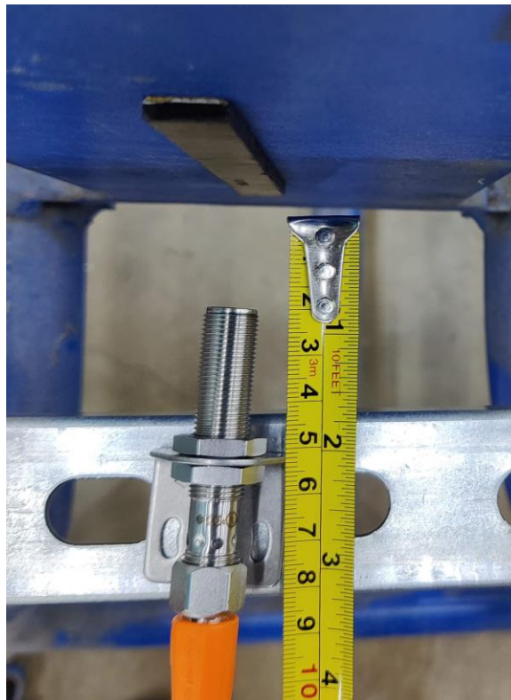
Figure 117: Mounting Proximity Sensor Assembly (Example)
