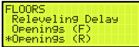
Figure 155: FLOOR Menu – Openings
