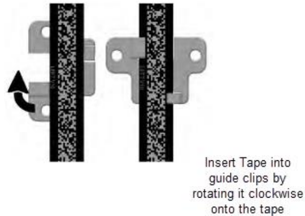
Figure 96: Tape Clip Insertion
