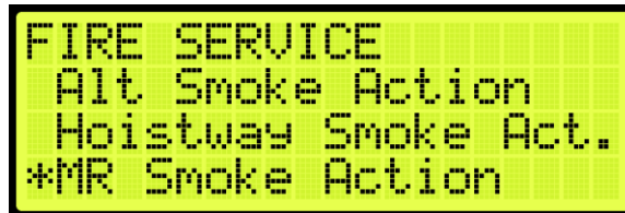
Figure 545: FIRE SERVICE Menu – MR Smoke Action
