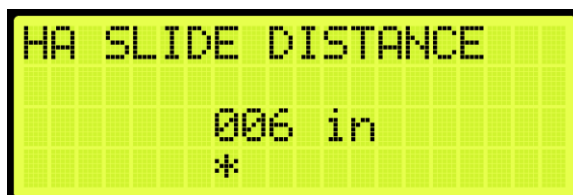
Figure 411: Hoistway Access Slide Distance
