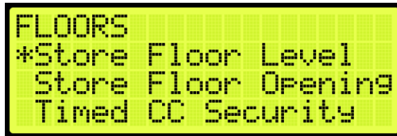
Figure 159: FLOORS Menu – Store Floor Level
