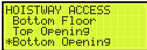
Figure 408: HOISTWAY ACCESS – Bottom Opening
