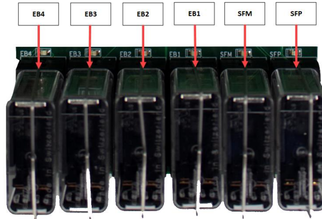
Figure 23: MR Board SR3032 Safety Relays
