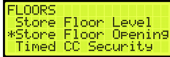
Figure 260: FLOORS Menu – Short Floor Opening
