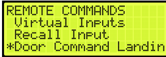
Figure 679: REMOTE COMMANDS Menu – Door Command Landing
