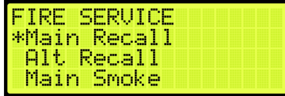
Figure 557: FIRE SERVICE Menu – Main Recall
