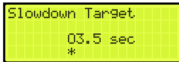
Figure 360: Slowdown Target- Increase
