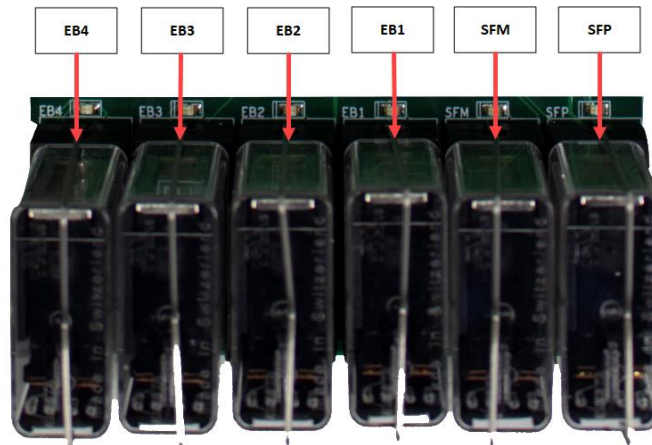
Figure 23: MR Board SR3032 Safety Relays
