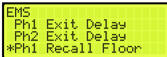
Figure 591: EMS Menu – Ph1 Recall Floor
