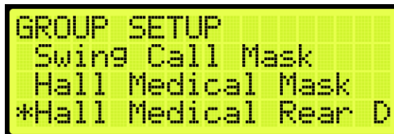
Figure 295: GROUP SETUP Menu – Hall Medical Rear Door Mask
