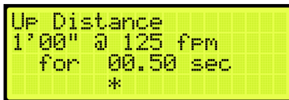
Figure 356: Up Distance Menu – Steady State of Leveling Longer Adjustment
