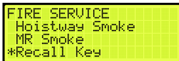
Figure 550: FIRE SERVICE Menu – Recall Key
