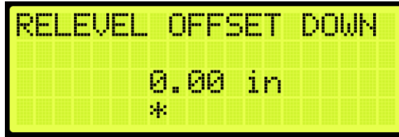
Figure 342: Relevel Offset Down Menu
