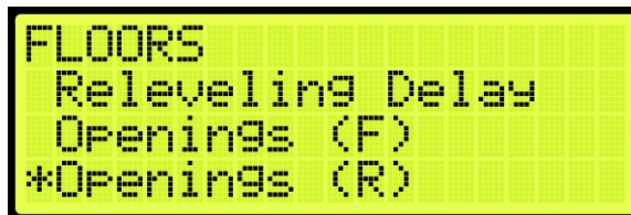
Figure 155: FLOOR Menu – Openings
