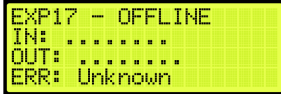
Figure 609: Inactive Expansion Board Status
