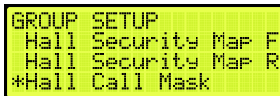
Figure 289: GROUP SETUP Menu – Hall Call Mask
