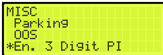
Figure 444: MISCELLANEOUS Menu – Enable 3 Digit PI
