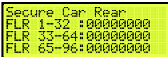
Figure 629: Secure Car Rear Menu
