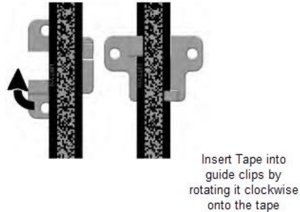
Figure 168: Tape Clip Insertion
