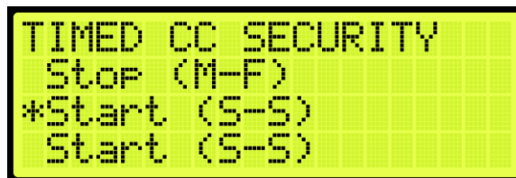
Figure 268: TIMED CAR CALL SECURITY Menu – Start (S-S)
