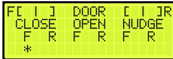
Figure 710: Enter Door Command Menu (Front and Rear Doors)
