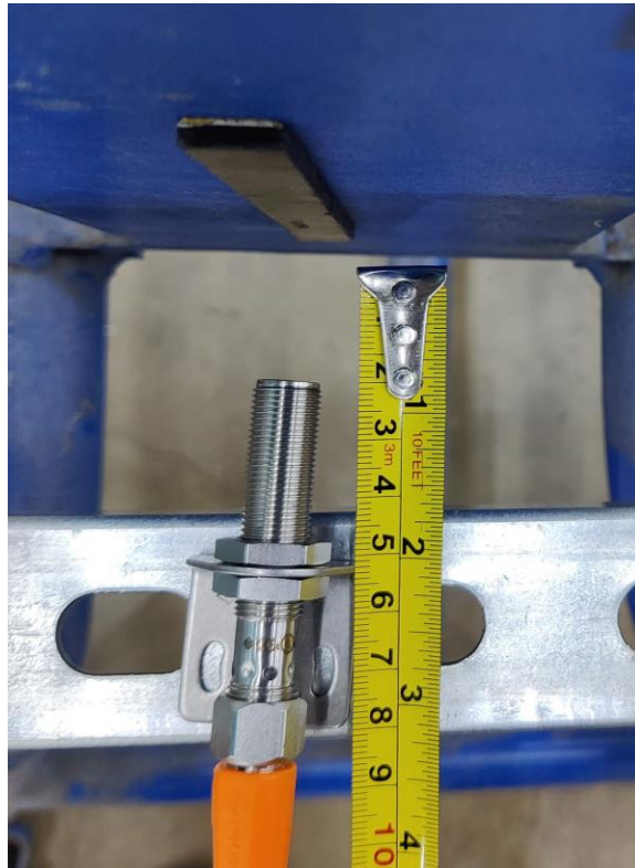
Figure 189: Mounting Proximity Sensor Assembly (Example)
