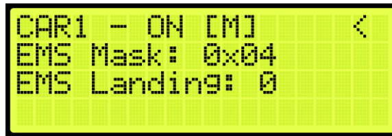
Figure 377: Emergency Medical Call Mask and Landing
