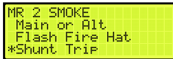
Figure 615: MR 2 SMOKE Menu – Shunt Trip
