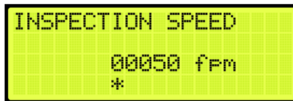
Figure 125: INSPECTION SPEED Menu
