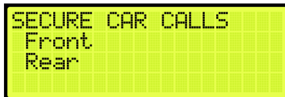
Figure 666: SECURE CAR CALLS Menu – Front or Rear
