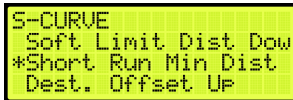
Figure 146: S-CURVE Menu – Short Run Min Distance
