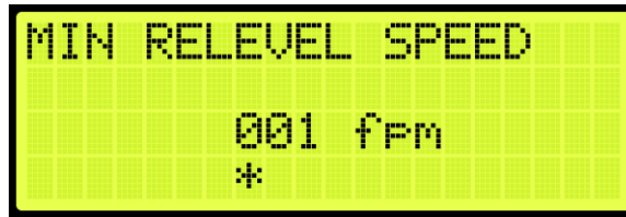
Figure 223: MINIMUM RELEVEL SPEED Menu
