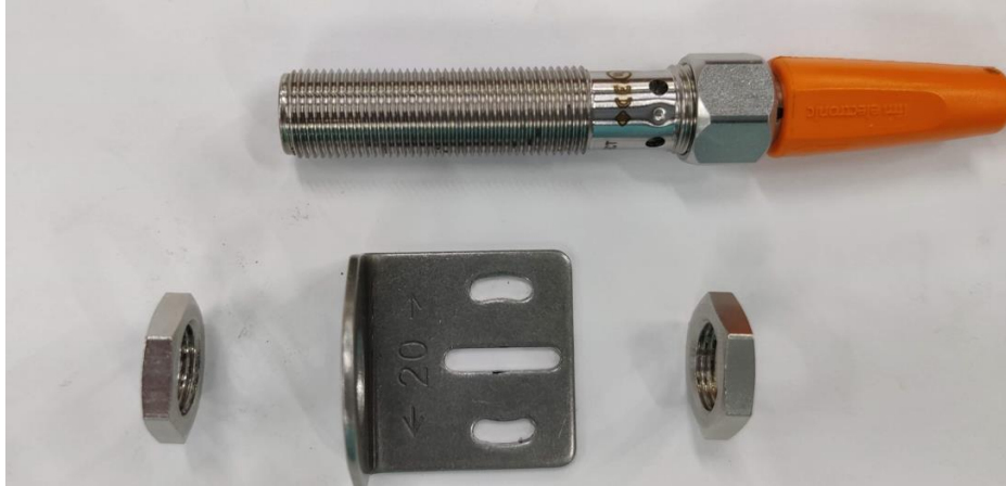
Figure 188: Proximity Sensor Assembly
