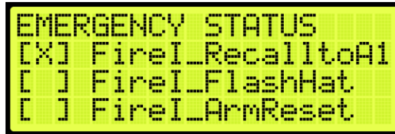
Figure 715: EMERGENCY STATUS Menu
