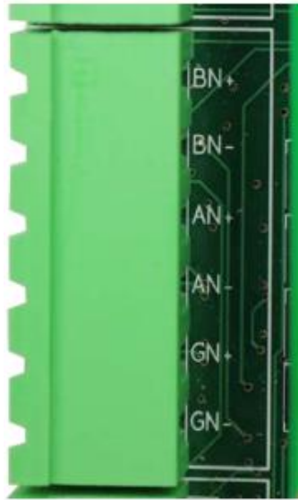
Figure 14: CAN 1,2,3 Network Connector
