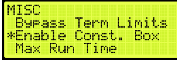
Figure 428: MISCELLANEOUS Menu – Enable Construction Box
