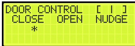
Figure 711: Enter Door Command Menu (Front Doors Only)
