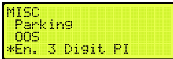
Figure 458: MISCELLANEOUS Menu – Enable 3 Digit PI
