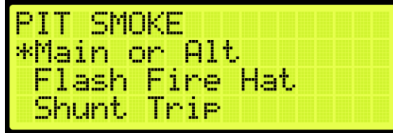
Figure 597: PIT SMOKE Menu – Main or Alt
