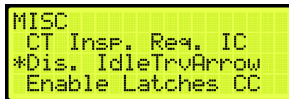
Figure 434: MISCELLANEOUS Menu – Disable IdleTrvArrow
