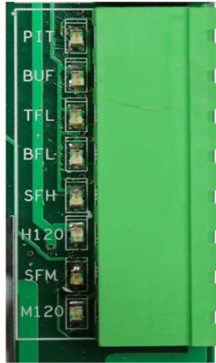
Figure 19: Safety String Input Connector
