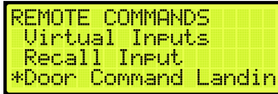
Figure 677: REMOTE COMMANDS Menu – Door Command Landing
