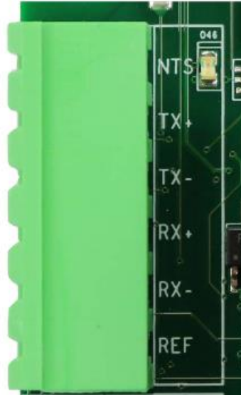
Figure 12: Drive Communication Connector
