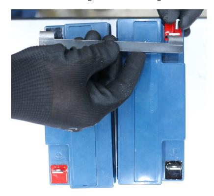
Figure 12: Bus Bar Holding Two Batteries
