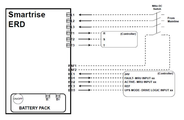
Figure 6: ERD External Wiring
