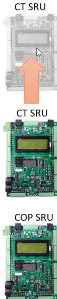
*Figure 10: Replacing MR SRU with CT SRU*
