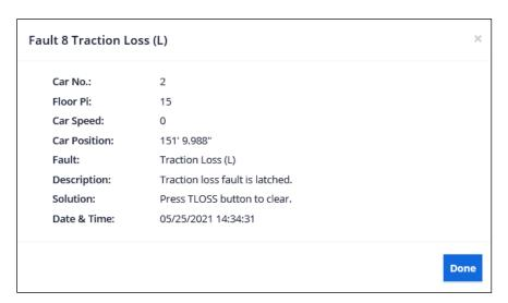
Figure 26: Fault and Traction Loss Pop-up
