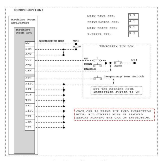
Figure 4: Example of Construction Wiring
